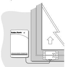
Open the door or window. The light on the sensor transmitter turns on each time you open the door or window.
